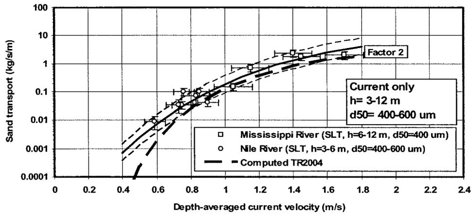
Fig. 4. Suspended transport as function of current velocity for  $d_{50}=400\text{--}600\ \mu\text{m}$ ; river and tidal flow
