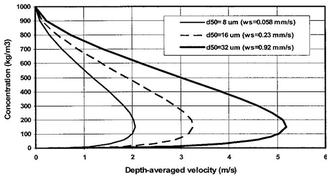
**Fig. 21.** Saturation concentration as function of depth-averaged velocity and particle size of fine sediments ( $h=10$  m,  $C=100$  m<sup>0.5</sup>/s,  $c_{\max}=1,000$  kg/m<sup>3</sup>,  $\nu=10^{-6}$  m<sup>2</sup>/s)
