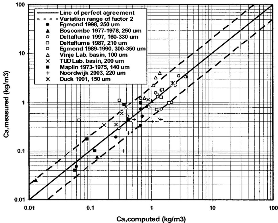
Fig. 16. Measured and computed reference concentrations for 54 cases
