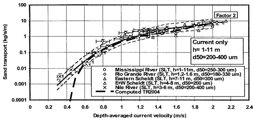
Fig. 3. Suspended transport as function of current velocity for  $d_{50}=200\text{--}400\ \mu\text{m}$ ; river and tidal flow
