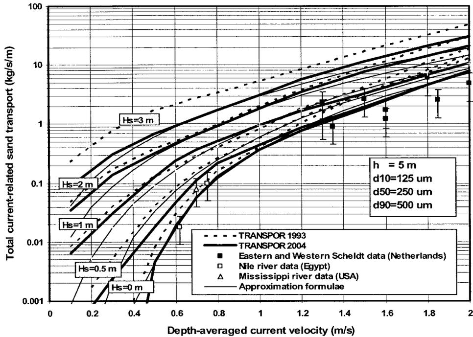
Fig. 20. Total sand transport for combined wave-current conditions,  $h=5$  m,  $d_{50}=250$   $\mu$ m
