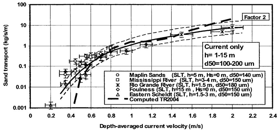
Fig. 2. Suspended transport as function of current velocity for  $d_{50}=100\text{--}200\ \mu\text{m}$ ; river and tidal flow
