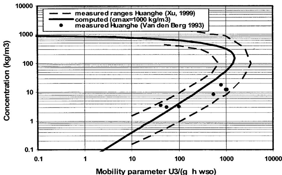
**Fig. 22.** Saturation concentration as function of dimensionless mobility parameter ( $h=10$  m,  $C=100$  m<sup>0.5</sup>/s,  $c_{\max}=1,000$  kg/m<sup>3</sup>,  $\nu=10^{-6}$  m<sup>2</sup>/s)
