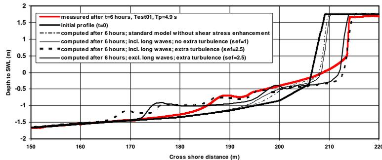
Figure 2 Computed bed profiles after 6 hours for Test T01
