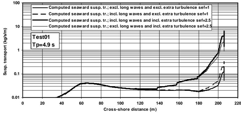
Figure 4 Computed seaward suspended sand transport for test T01 (at t=0 hrs)
