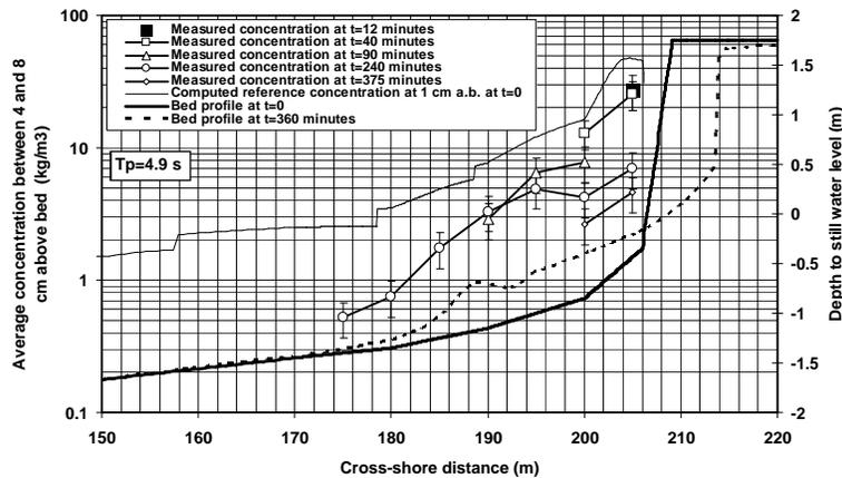
**Figure 3** Measured and computed reference concentration for Test T01
