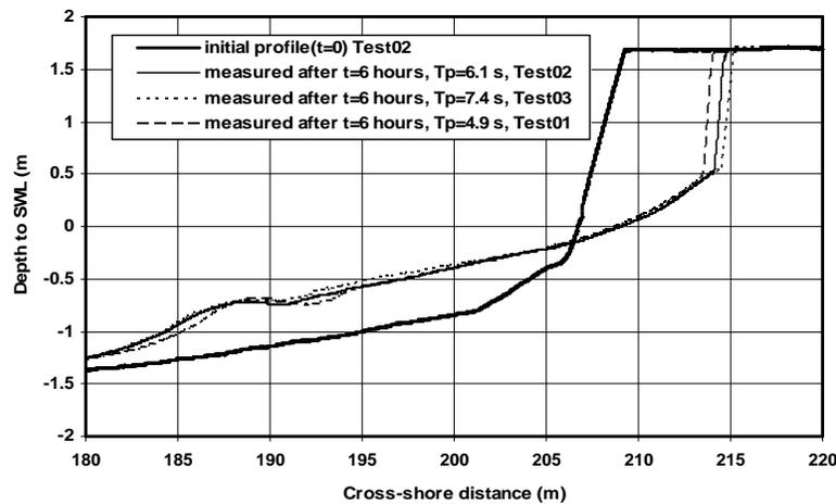
Figure 1. Measured bed profiles after 6 hours for Tests T01, T02 and T03
