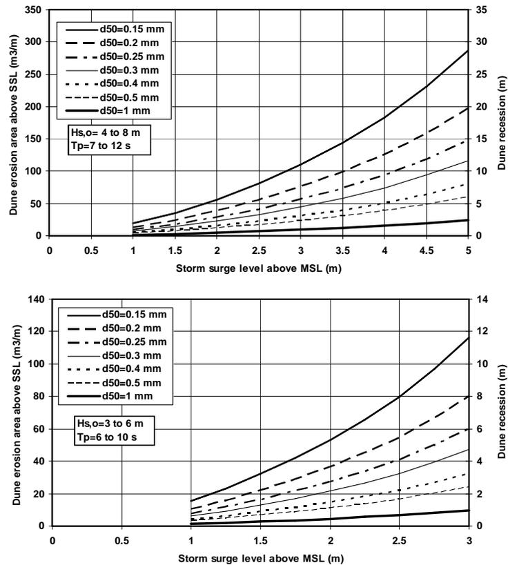
Figure 6 Dune erosion after 5 hours as function of sediment size and storm surge level for two wave climates: North Sea (upper) and Mediterranean (lower); dune recession based on dune height of 10 m above SSL
