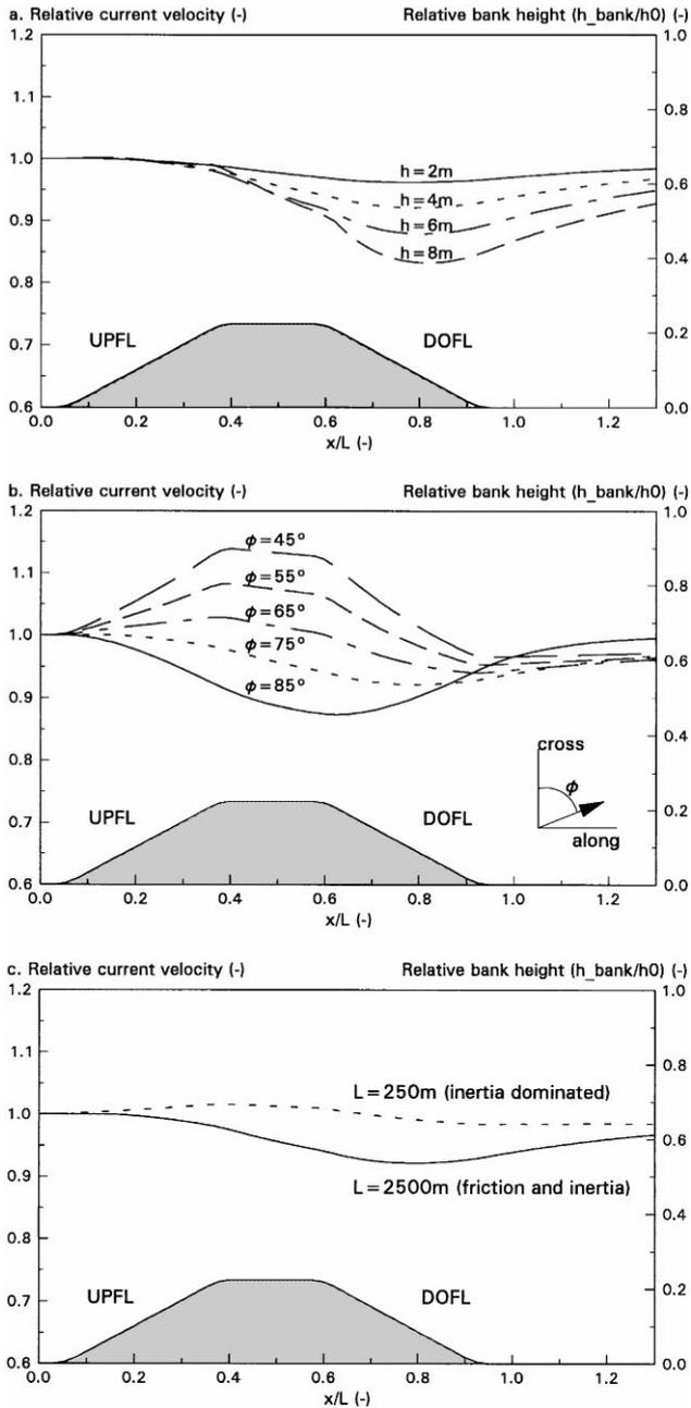
Fig. 6. Sensitivity analysis *Trenchflow*. Reference conditions as in Fig. 5. (a) Flow response (total velocity vector) as a function of sand bank height  $h_{\text{bank}}$ ; (b) flow response as a function of sand bank orientation with respect to the undisturbed flow  $\phi_0$ ; and (c) flow response as a function of sand bank wavelength  $L$ . Summary of input conditions given in Table 1.
