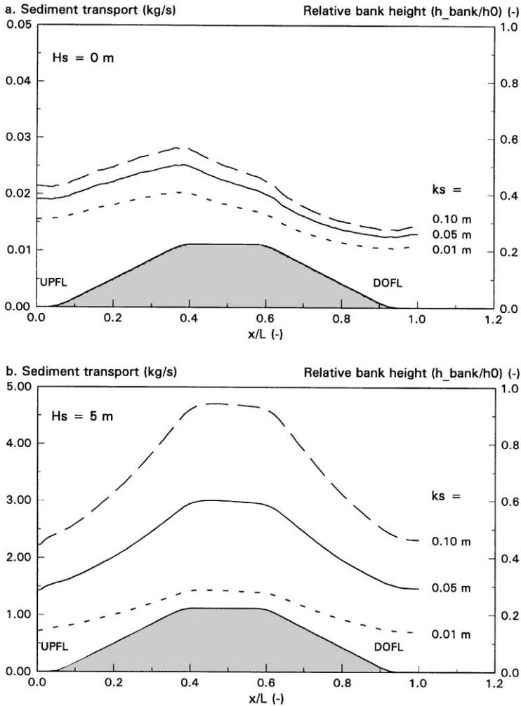
Fig. 8. Sediment transport rates across a linear sand bank calculated with *Sutrench*. Input is the flow response given in Fig. 5 (reference conditions for a typical spring tidal flood current). UPFL = up-current flank, DOFL = down-current flank. (a)  $H_s = 0$  m,  $k_s = 0.01, 0.05, 0.10$  m; (b)  $H_s = 5$  m,  $k_s = 0.01, 0.05, 0.10$  m.
