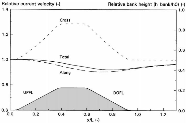
Fig. 5. Flow response across a linear sand bank. Reference conditions typical for a spring tidal flood current ( $U_0 = 0.8$  m/s,  $\phi_0 = 75^\circ$ ,  $L = 2500$  m,  $h_{\text{bank}} = 4$  m,  $h_0 = 18$  m,  $k_s = 0.05$  m; UPFL = up-current flank, DOFL = down-current flank).
