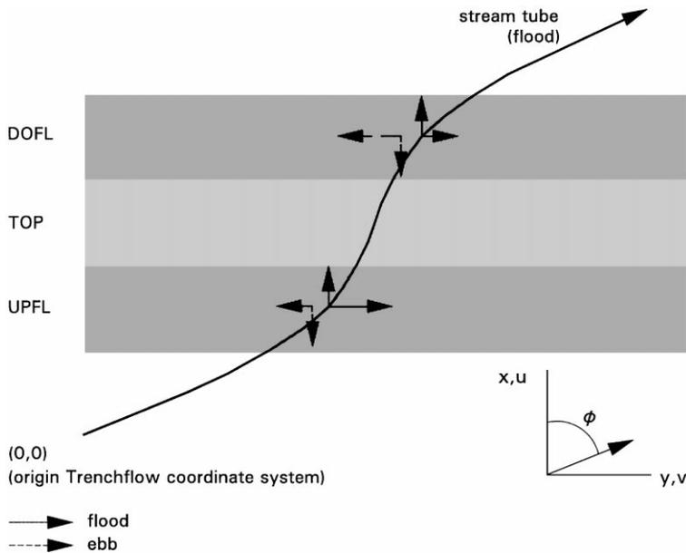
Fig. 2. Coordinate system *Trenchflow* (after Boer, 1985). UPFL = up-current flank; TOP = top of the ridge; and DOFL = down-current flank.
