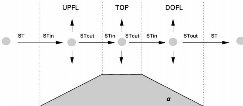
Fig. 4. Definition of the sand bank topography used for the *Sutrench* calculations: UPFL = up-current flank; TOP = top of the ridge; DOFL = down-current flank; and ST = total sediment transport.
