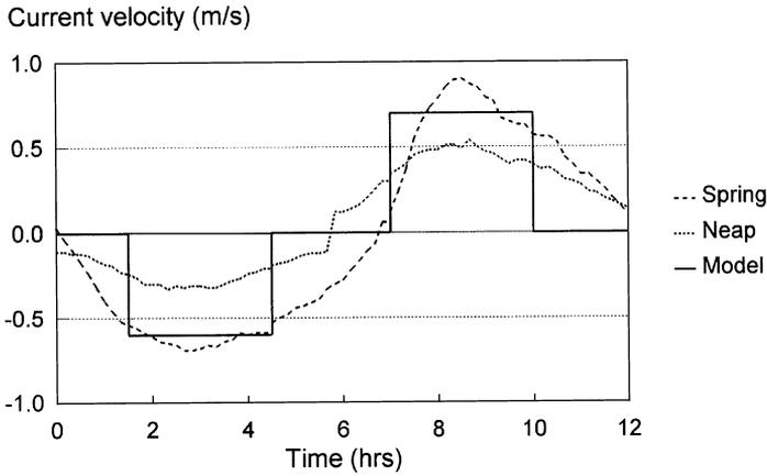
Fig. 7. Characteristic tidal velocity curve and schematized velocity regime. Positive is flood; negative is ebb.
