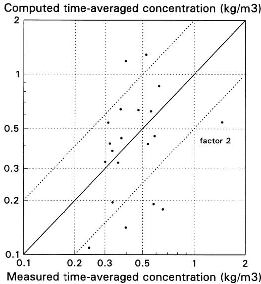
Fig. 3. Comparison between observed and computed near-bed sediment concentrations during a storm.
