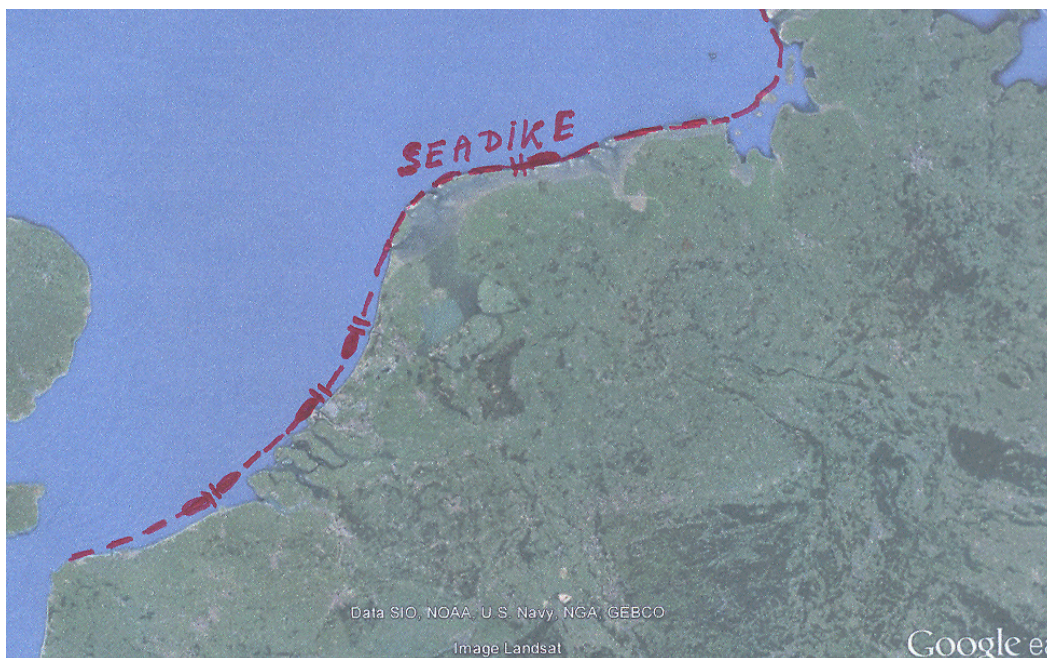
Figure 6 Offshore seadike in the case of excessive Sea Level Rise > 5 m (sluice systems and offshore islands for ports/airports are included)
