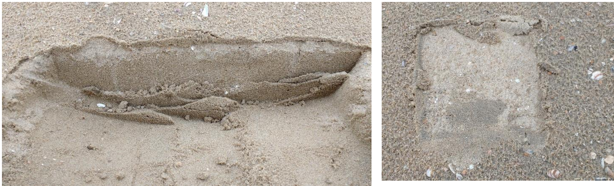
Figure 5 Beach surface immediately after rainfall in winter; 8 February 2020; Callantsoog, Netherlands Left: vertical cut with moist top layer of 5 mm and dry layer of 10 to 15 mm; Right: moist layer is removed with spade showing dry sand surface beneath
