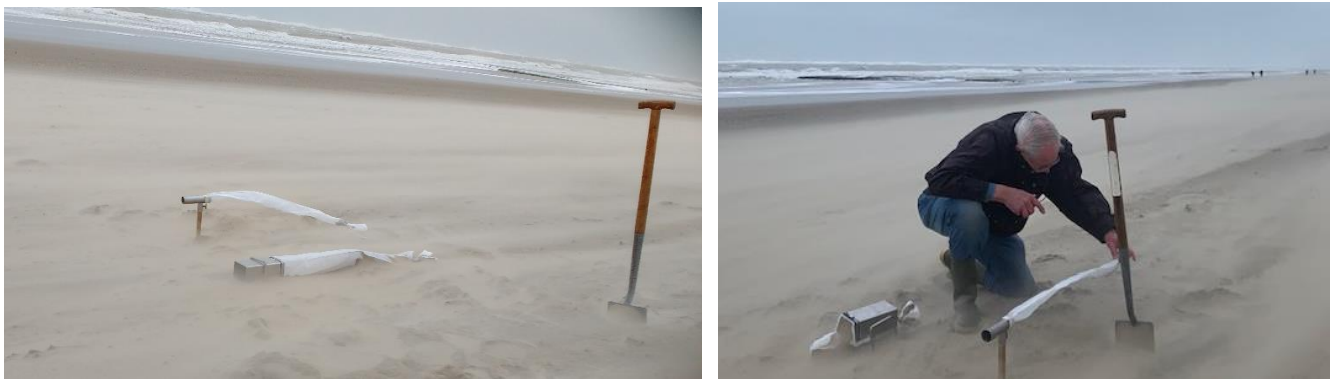
Figure 3 Wind transport at beach of Callantsoog; major storm BF 9 (18 m/s) on 9 February 2020 (lighter colours represent is a thin, dense layer of saltating grains with continuous transport)
