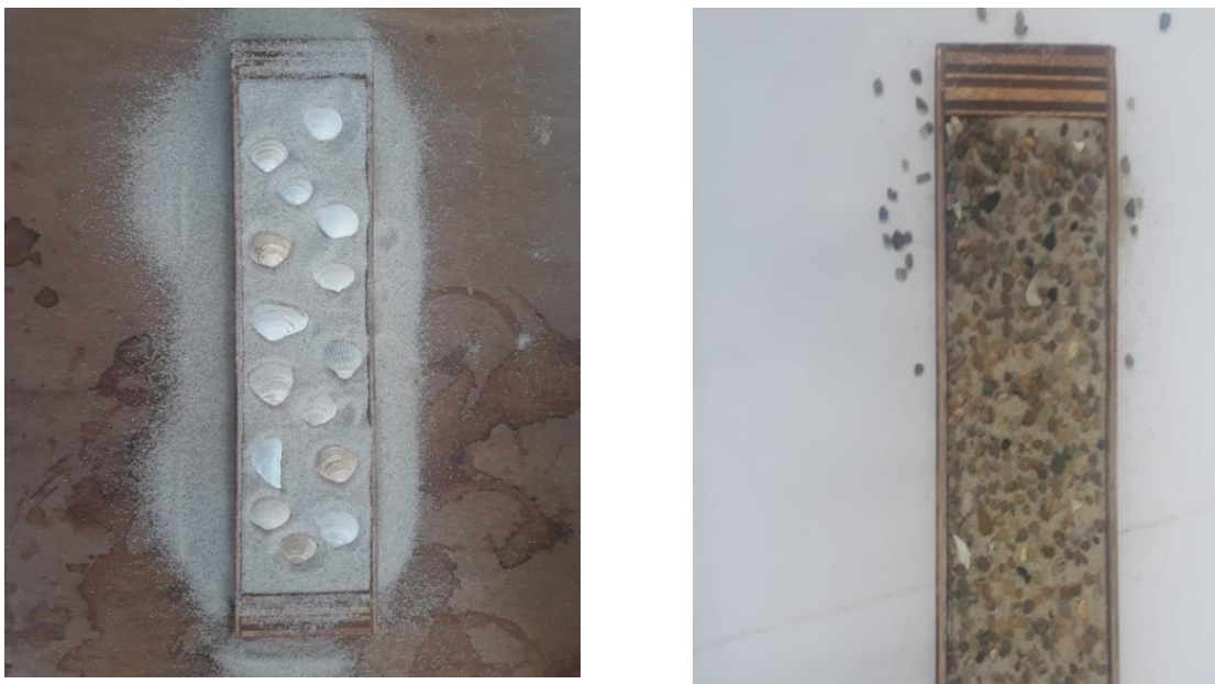
Figure 13 Laboratory setup with shells and gravel in tray of mini wind tunnel (length of tray=250 mm)
