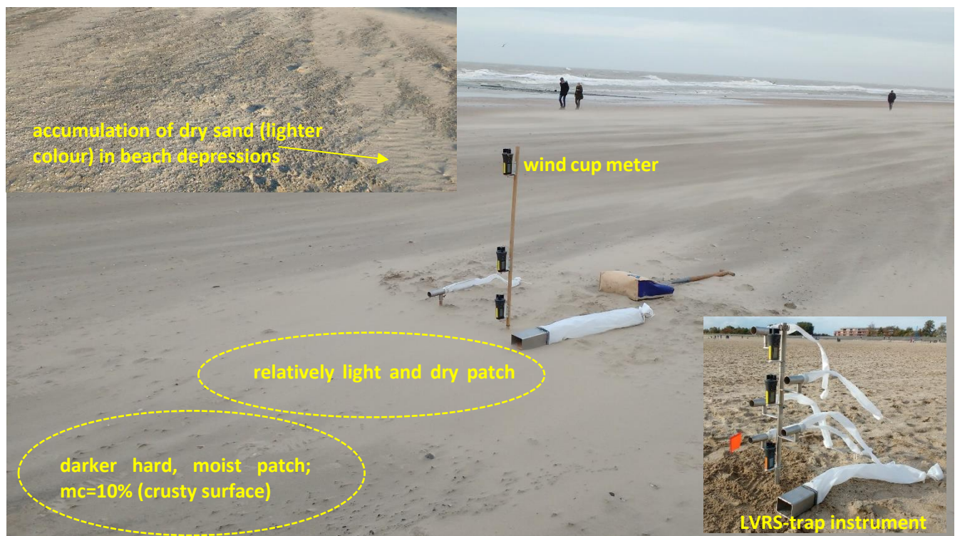
Figure 1 Wind transport at beach of Callantsoog; minor storm BF 6/7; 15 February 2020 (mc=moisture content)
