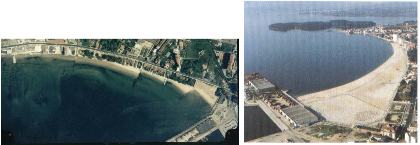
Figure 1.2 Example of the removal of a coastal groin system in Compostela beach (Spain) before (left) and after beach restoration (right); fill nourishment is included.
