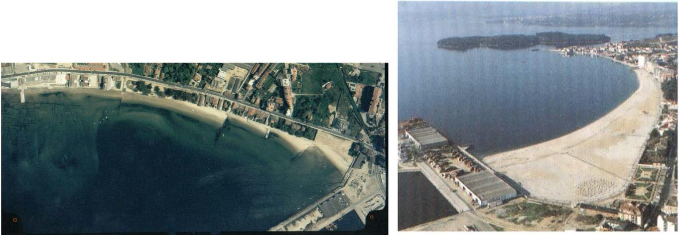
**Figure 2** Example of the removal of a coastal groin system in Compostela beach (Spain) before (left) and after beach restoration (right); fill nourishment is included.
