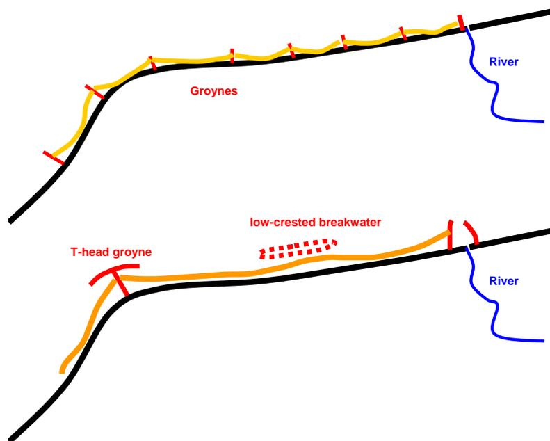
**Figure 3.** *Long, wide beach replacing small cell-type beaches*
