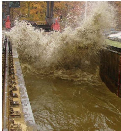
Figure 1B Impact of incoming and outgoing (reflected) waves in Deltaflume
