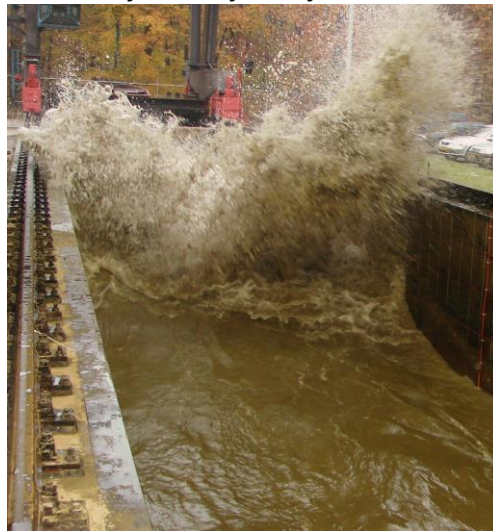
Figure 1B Impact of incoming and outgoing (reflected) waves in Deltaflume
