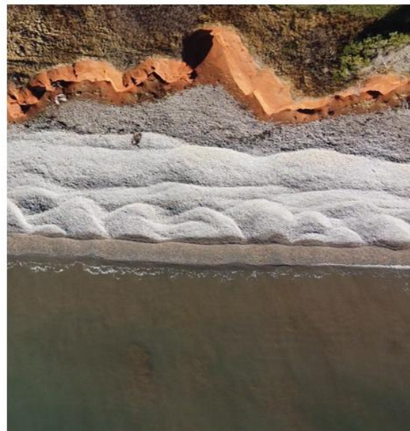
Figure 7.2.4 Beach nourishment of coarse sediments ( d_{50}\geq 40 mm) pebbles, Magdalen Island
