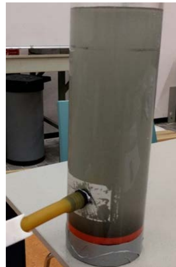
Figure 12 Sampling tube and settling column for in-situ settling velocity (WASED; www.wiertsema.nl )
