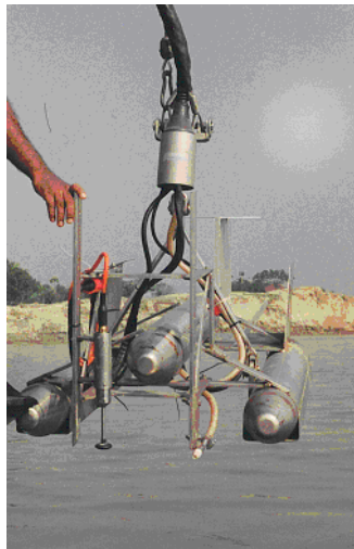
Figure 9 Instrument carrier with pump intake nozzle, current meter, echo-sounder or pressure sensor for vertical position.
