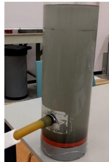
Figure 5.12 Sampling tube and settling column for in-situ settling velocity (WASED; www.wiertsema.nl )
