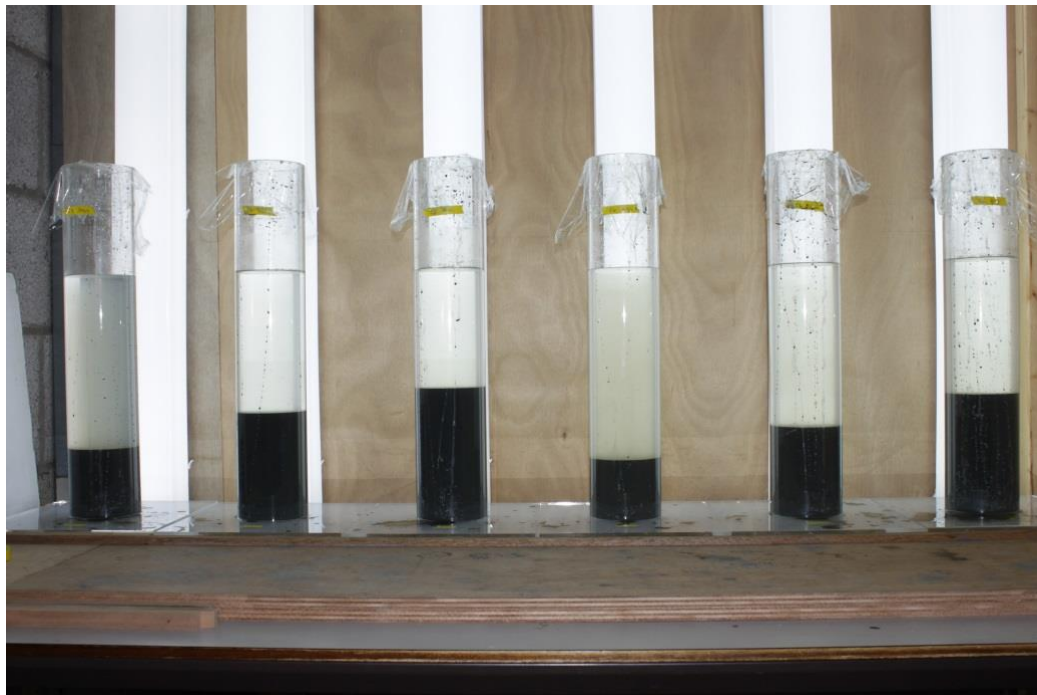
Figure 5.9 Settling tests using perspex tubes/columns
