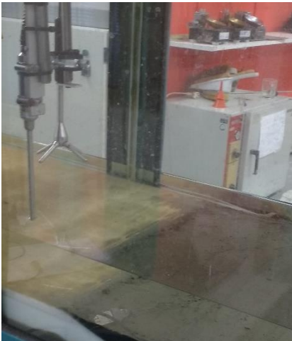
Figure 5.17 Flume setup for critical bed-shear stress of mud-sand beds
