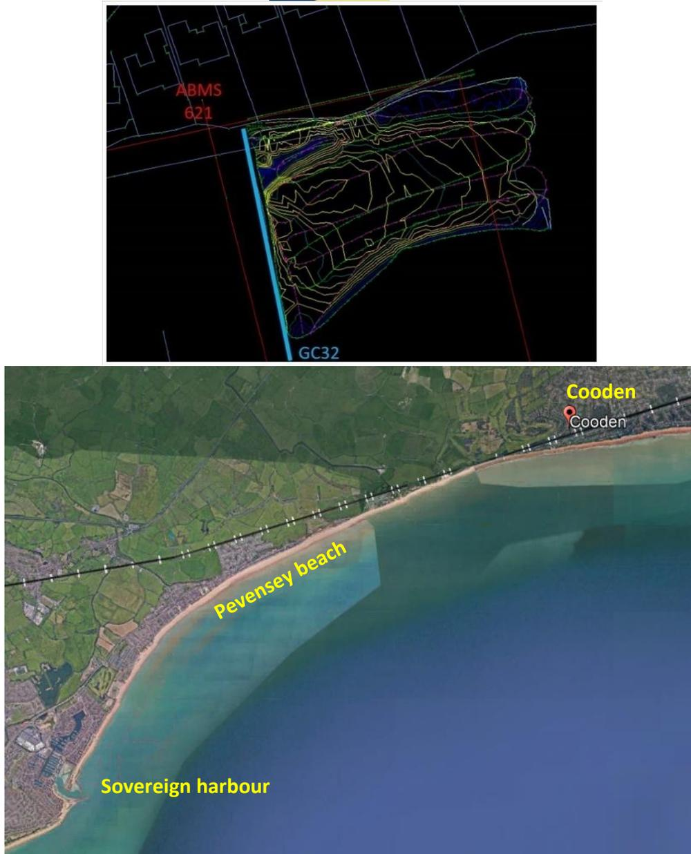
**Figure 4.4.3** Beach level changes (1-3 November 2023) east of terminal groyne GC32 at Cooden (Pevensey beach, UK) after storm Ciaran (blue=loss of sediment  $\cong 120 \text{ m}^3$ ; Yellow=gain of sediment  $\cong 1880 \text{ m}^3$ )
