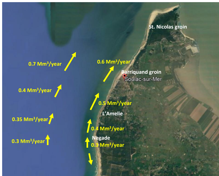
Figure 3.6.4 Net annual longshore sand transport values in shoreface zone (seaward of -5 m depth) and in surf zone (landward of -5m depth line)
