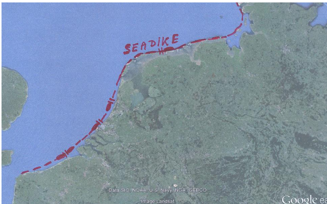
Figure 5.5 Offshore sea dike in the case of excessive sea level rise of 2 to 10 m (sluice systems and offshore islands for ports/airports are included)
