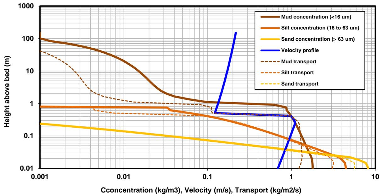
Figure 4.1 Sediment concentrations and transport of example computation
