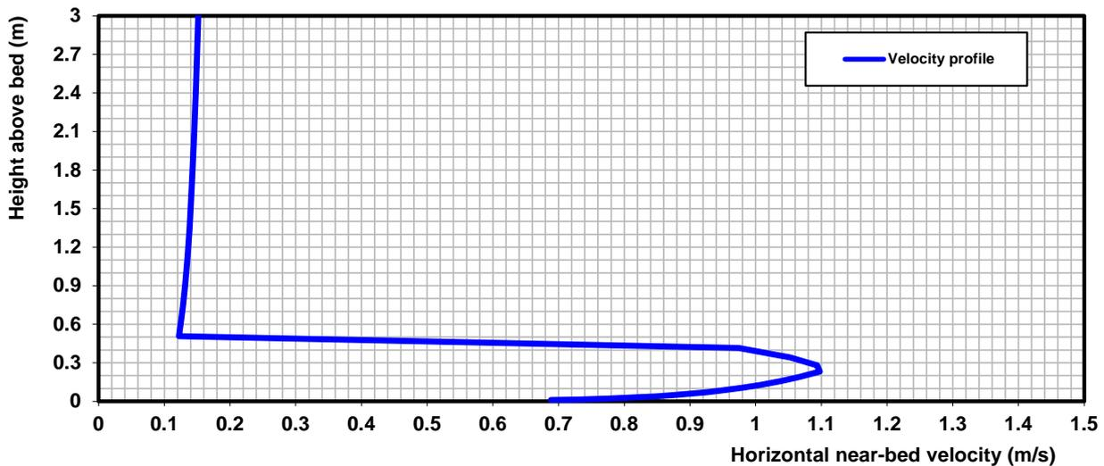
Figure 2.1 Flow velocity profile ( $u_{\max} = 1 \text{ m/s}$ ,  $\delta = 0.5 \text{ m}$ ,  $u_{\text{mean}} = 0.2 \text{ m/s}$ ,  $h = 150 \text{ m}$ ;  $k_{s,c} = 0.01 \text{ m}$ )
