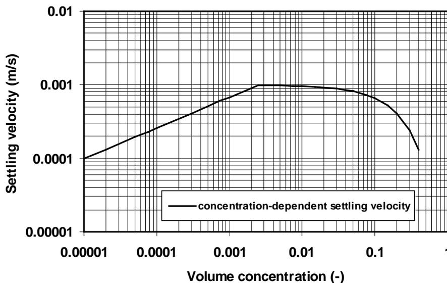
**Figure 3.1** Settling velocity as function of volume concentration; flocculation range for  $c < 0.0025$  and hindered settling range for  $c > 0.0025$ ;  $w_{\text{mud,max}} = 0.001$  m/s,  $w_{\text{mud,min}} = 0.0001$  m/s
