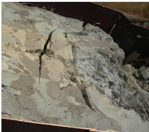
Figure 2.2.3 Dutch boulder clay (upper: excavation at local dike; lower: tests in Delta flume)
