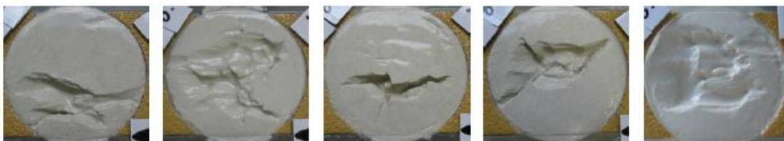
Figure 2.3.3 Examples of eroded surfaces with cracks (Jacobs 2011)
