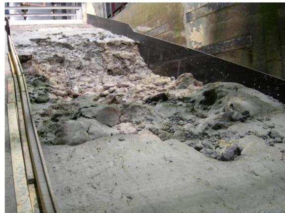
Figure 2.2.3 Dutch boulder clay (upper: excavation at local dike; lower: tests in Delta flume)
